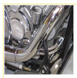
11. Complete the installation by filling engine with specified amount of oil as shown in Yamaha shop manual. Start engine, check for leaks, turn off engine and recheck oil level. Add oil as needed to achieve correct level.
