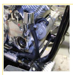
7. Install the new oil relocation assembly by sliding the diverter between the down tubes of the frame and the front of the engine taking care to protect the part from contacting the frame or motor as seen:
