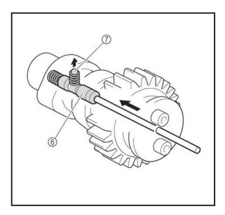
The decompression cam (6) is pushed in the direction indicated by the arrow, and then the pin (7) raises the projection of the decompression cam.
